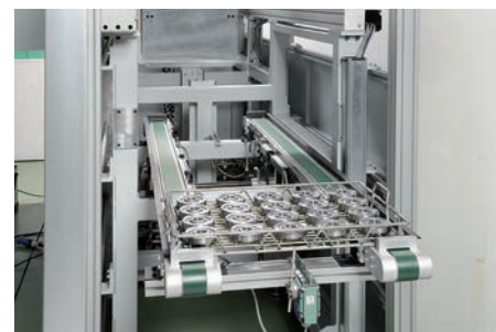
Basket positioned for loading or unloading from a robot or a gantry. Two or more loading or unloading areas can be supplied.
